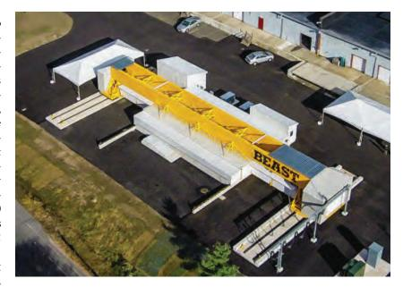
The BEAST is composed of a set of parallel steel I beams 120 ft long by 7 ft deep, steel-framed end towers, and concrete abutments approximately 15 ft tall.
