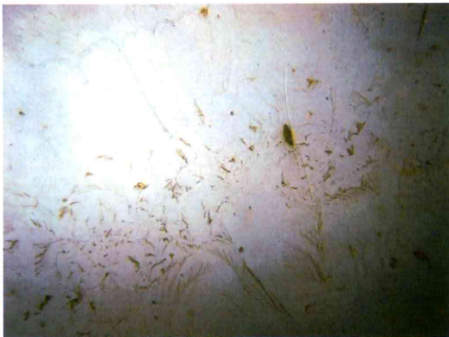
39 Floor Surfaces Found With Coating Failure, Exposed Steel, Moderate Surface Corrosion And Pitting After Cleaning
